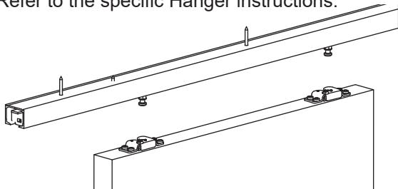
(b) Adjust the height to make sure the clearance between panel and track are in specification as shown below.
