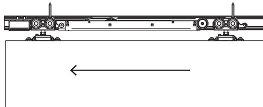
(b) Slowly move the panel to the open position and the soft close should be primed and ready for use.
