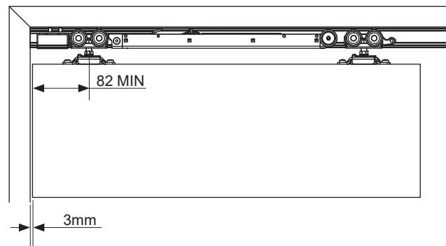
(b) Adjust the position of the Catch Plate as necessary to achieve the 3mm.
