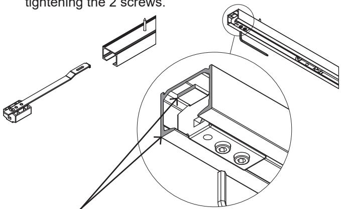
(b) Ensure the end of the plate and the end of the track are aligned, (shown in grey).
